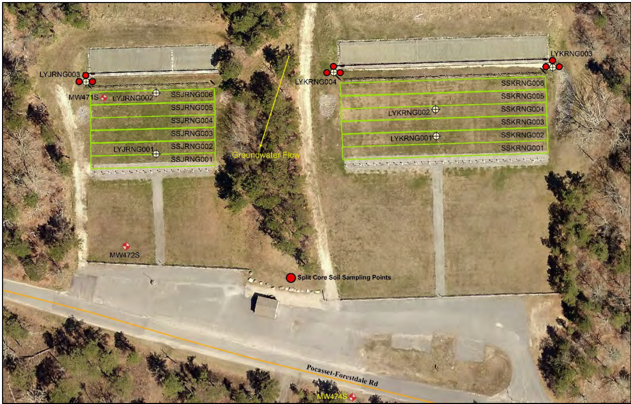
Juliet and Kilo Ranges, STAPP bullet catcher system, Camp Edwards, Massachusetts LY=Lysimeter, MW=Monitoring Well, SS=Soil Sample
