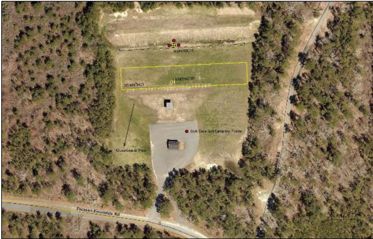
India Range, Copper Ammunition Only, Camp Edwards, Massachusetts. LY=Lysimeter, MW=Monitoring Well, SS=Soil Sample
